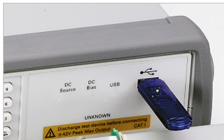
Figure 6. Example of use with USB storage device
